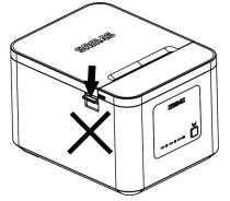
2) Fix the printer by one hand and press either side of the convex bars by the other hand. Push up and open the front cover.
