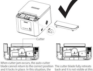
blade cannot return to the correct position The cu and it locks in place. In this situation, the roll paper cover does not open even if you pull cover open lever. Figure 1
